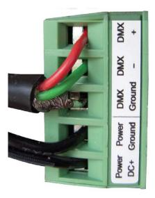
**DMX**: Connect the DMX cable to the lighting receivers (Leds, Dimmers, Fixtures..) [For XLR: 1=ground 2=dmx-3=dmx+)
